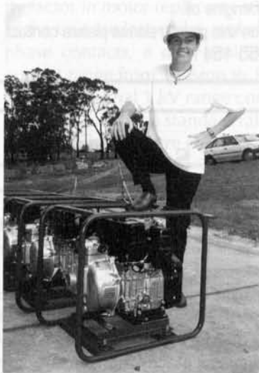
The diesel powered Fire Chief is suitable for tanker applications or as stand-by firefighter for mine sites
